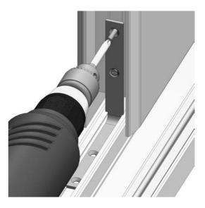
Ensure that the fixed patio sash is tight against the right hand outer frame then permanently secure the Fixed Pane Cleat (PT12) to the patio outer frame by use of the 4.3 x 30mm Patio Screws (PT5).
