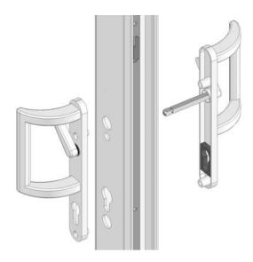
Place the external patio handle set against the external face of the sliding patio sash so that the spindle detail locates over the protruding Spindle (PT17e).
