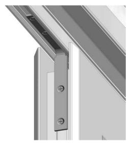
Reattach the Interlock (PT11) to the left face of the fixed sash by locating the right hand leg detail into the fixed patio sash.
