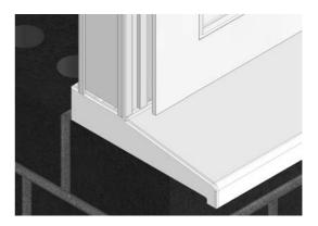
Locate the patio outer frame position by ensuring that the internal face of the patio outer frame is in line with the internal face of the 150mm sill (P106).
