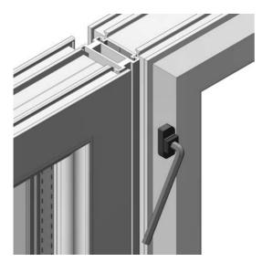
When the quarter turn button (C105) is in position and resting against the 18mm inline coupling (A104), turn the 6mm Allen key (6AK) 90° clockwise. The quarter turn button (C105) will 'click' into position.
