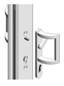
Slide the Barrel Lock (PT17f) through the barrel lock detail on each patio handle set ensuring that it is central to the width of the sliding patio sash.
