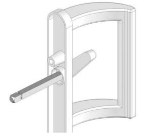
Place the internal patio handle set against the internal face of the sliding patio sash so that the Spindle (PT17e) locates into the spindle hole.
